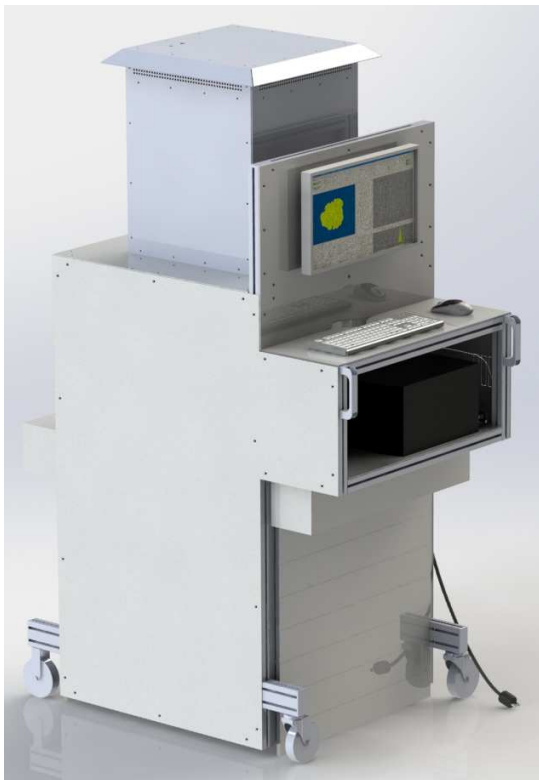
Figure 1. CropReporter for top view imaging of plants. Using high intensity red light emitting diodes fluorescence images are being captured, white light emitting diodes together NIR lighting are being used for spectral imaging at six different filter bands. Images are captured at a resolution of 1.4 Mp and 14 bit digital grey values.
