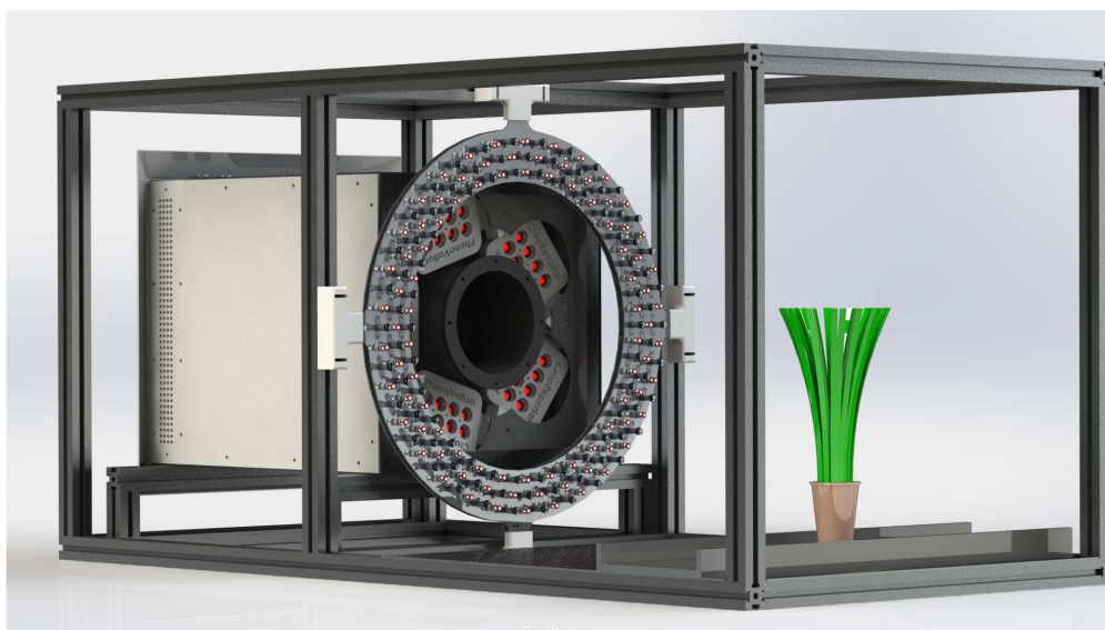
Figure 1. CropReporter for side view imaging of monocotyledons. Using high intensity red light emitting diodes fluorescence images are being captured, white light emitting diodes together NIR lighting are being used for spectral imaging at six different filter bands. Images are captured at a resolution of 1.4 Mp and 14 bit digital grey values.
